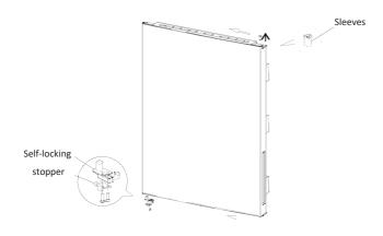
6)Remove the center hinge, then remove the center hinge shaft with a slotted screwdriver. Install the hinge shaft on opposite side of the hinge and install the hinge to the left of the box.
