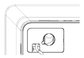
6-Mount Ice Maker to the two screws (#9) you started earlier from Step 3. Tighten screws (#9).
