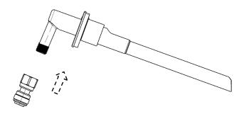
11. Push water inlet tube (#6) through small hole where Installation label was. Rotate while inserting tube until flat surface of inlet tube is tight against back of refrigerator., and finally make the limit fall on the limit hole.
