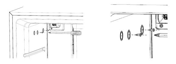
4. Connect the ground terminal first, then connect wiring harness into connector mounted on the back freezer panel, and make sure that the terminal buckle is installed in place
