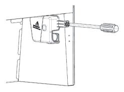
14. Use a flat-blade screwdriver to pry open the protection cover of the water valve, and take out the terminal protection box.
