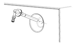
12. Use a Phillips screwdriver to fix the water inlet tube (#6) with the two fixing screws (#10), and check whether it is tightened.
