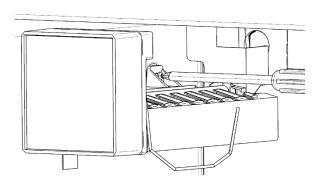
7. Put the freezer wire shelf on the middle floor, and place the ice container(#3) on the freezer wire shelf
