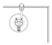
13. Use a Phillips screwdriver to remove the fixing screws (#11) and remove the back water valve protection box and protection cover.
