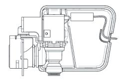
16. Assemble the water valve protection cover .
