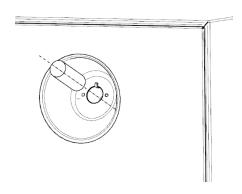
9. Paste two tybe seals(#7,#8) on the water supply pipe of the ice maker, pay attention to whether the paste is in place
