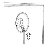
19. Use two pipe clamps (#4) (with adhesive surface) to organize the back water supply tubing(#5).
