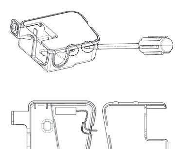
15. Connect the water (#2) valve terminal , pay attention to confirm whether the terminal buckle is installed in place, and put the terminal back to its original position in the protection box . Install the water valve into the water valve protection box.
