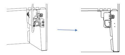
The white sponge should be reinstalled to prevent the cold air leakage.
