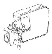
17. Use three screws (#11) to fix the water valve and the water valve protection box to the rear panel.
