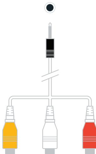
Connect a composite video cable and left-right audio cables from an external AV device.
