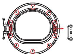
7. Remove the 8 screws from the inner door and rotate the rest parts for 180 degrees.
