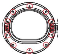
9. Install the door on the frame-front and then fasten the 2 screws that were removed in Step 2.
