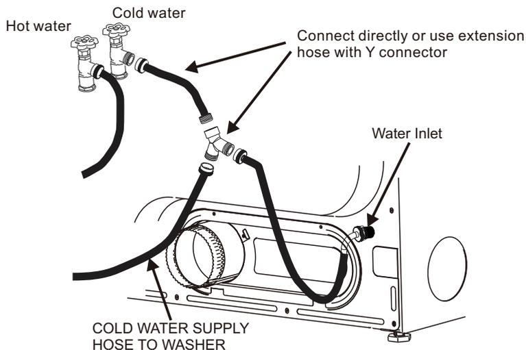
If possible install the “Y” connector directly, thread the short extension hose onto the COLD water supply and snug it by hand; then tighten it another  $\frac{2}{3}$  turn with pliers. Thread the “Y” connector to the short extension hose and snug it by hand; then tighten it another  $\frac{2}{3}$  turn with pliers.
