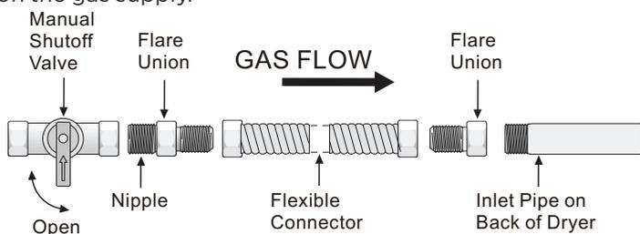
All connections must be wrench-tightened
