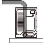
Clean all old ducts before installing your new dryer. Be sure the vent flap opens and closes freely. Inspect and clean the exhaust system annually.
