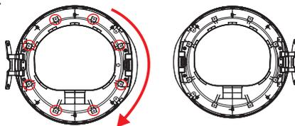
8. Assemble the inner door and the back cover, place the door pin on the opposite side and then fasten the 14 screws that were removed in Step 6.
