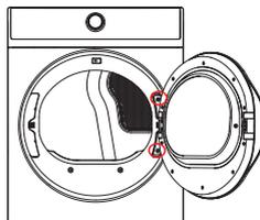
4. Using a flat-blade screwdriver, remove the hinge hole cover.
