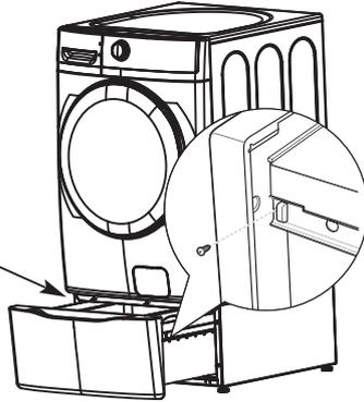
**C** Reinstall the original screws into each drawer slide. Tighten both screws.
