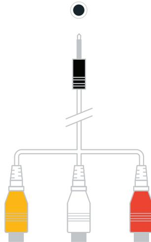
Connect a composite video cable and left-right audio cables from an external AV device (AV adapter included).
