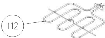
TOP AND GRILL HEATING ELEMENT (OPTIONAL ONLY FOR ELECTRIC GRILL NEW G.FS GAS)
