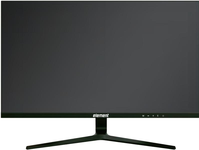
**Indicator Light** –the light is blue when the monitor is turned on. The light is off when the monitor is turned off. The light is red when there is no signal given to the monitor.
