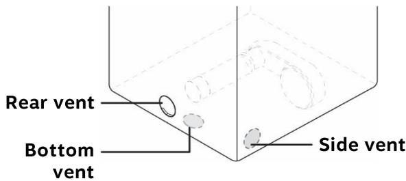
Adapter kits, which are standard components, can be purchased from any retailer. These kits contain the necessary duct components to change the dryer vent location.
