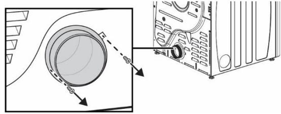
2. Press the tabs on the knockout and carefully remove the knockout for the desired vent opening.
