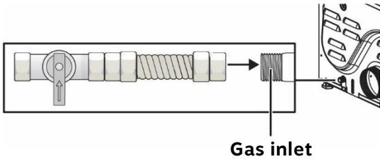
ⓘ An additional fitting is required to connect the 3/4 in. (1.9 cm) female thread end of a flexible connector to the 3/8 in. (1 cm) male threaded end on the dryer. Use only new AGA or CSA certified gas supply line with SS flexible connectors within 6 ft. (1.8 m) of the dryer.
