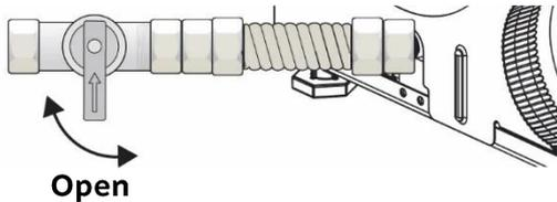
8. Check all gas connections for leaks using a soap solution. If bubbles appear, tighten the connections, and then recheck it.
