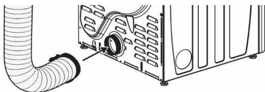
**i** For a tight installation, attach a section of the exhaust system onto your dryer before putting it in place.
