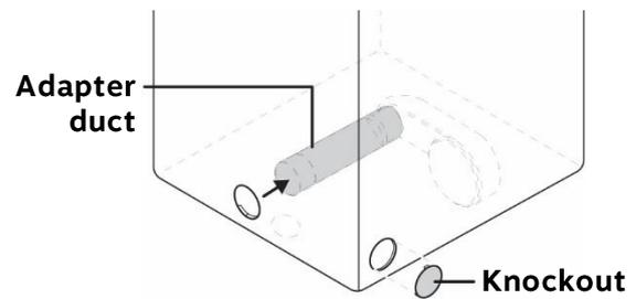
3. Attach the adapter duct onto the blower housing of the dryer.
