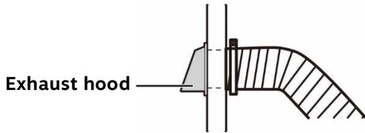
3. Connect the duct to the venting hole on the back, side, or bottom of the dryer and secure with aluminum tape. Do not cover the ventilation holes on the back of the dryer cabinet.
