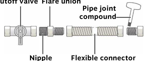
**i** The pipe joint compound must be resistant to the actions of any liquefied petroleum gas.
