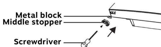
14. Align the middle hinge, making sure that the pin is in the hole on your refrigerator door, then secure in place with screws and a Phillips screwdriver.
