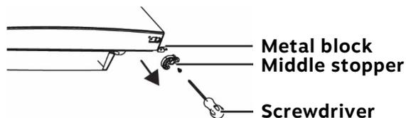
13. Install the middle stopper and metal block from your spare parts bag on the opposite side of the freezer door.
