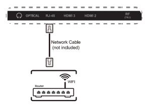
4. if you have a high-speed internet connection, connect a network cable from your modem/router to the back of the TV as shown.
